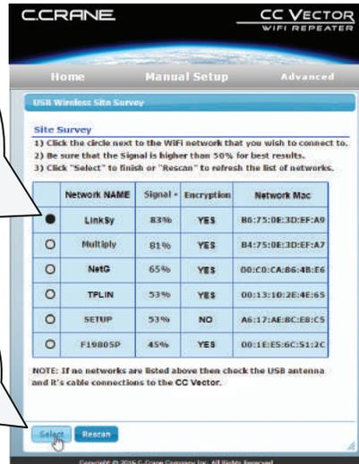
**NOTE:** For best performance, your signal should be higher than 50%. For a better signal, try adjusting the orientation and placement of the USB antenna - then click “Rescan” to see if the signal is higher.
