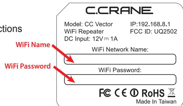
**C** After confirming you have completed Step “B”, open the Internet Browser screen on your device and enter **192.168.8.1** into the Address Bar. Press “Enter” on your keyboard.
