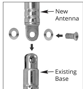
**Note: Opening the radio case will void your warranty.** The only part of the antenna that you need to replace is the visible portion from the pivot point up. If the bottom portion of the antenna is damaged, the radio will need to be sent in for repair.
